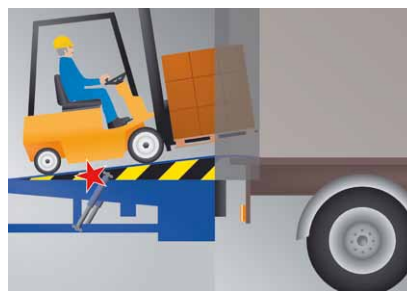
Safeguard emergency stop with two cylinders.
